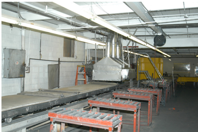
Fig. 1. Typical buffing line. Buffing wheel is located in the center of the hood. The extruded aluminum is placed on a table that traverses back and forth under the hood. Buffing compound is applied to the aluminum and the buffing wheel is then lowered against the surface of the material. (For interpretation of the references to color in this figure legend, the reader is referred to the web version of the article.)
