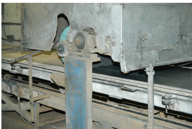
Fig. 2. Photograph of extruded aluminum traversing from left to right under buffing wheel and hood. A portion of bluish-green buffing wheel is visible in center of the picture. Tan colored buffing compound can be seen to the left of the buffing wheel, and the luster of the buffed aluminum surfaces can be seen to the right of the buffing wheel. (For interpretation of the references to color in this figure legend, the reader is referred to the web version of the article.)
